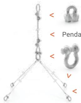
Forged wire rope clips for creating desired size top loops. Use 2 to insure safety.
